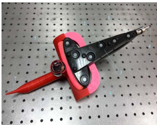
Figure 3. The working body for measuring the position and speed during manual movement: 1 – the probe of a stereophotogrammetric coordinate measuring machine; 2 – reflector; 3 – hard base; 4 – a spherical ruby tip of a stereo gram-metric machine; 5 – reflector of the coordinate measuring system; 6 – connecting equipment; 7 – the nozzle imitating the medical tool.
